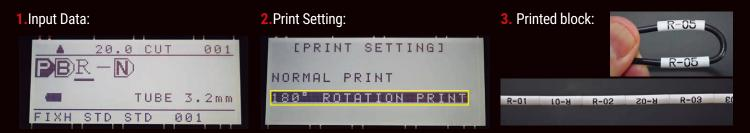
\*Marking blocks are automatically duplicated, the duplicated marking blocks can not seen if you press `IMAGE` key.
