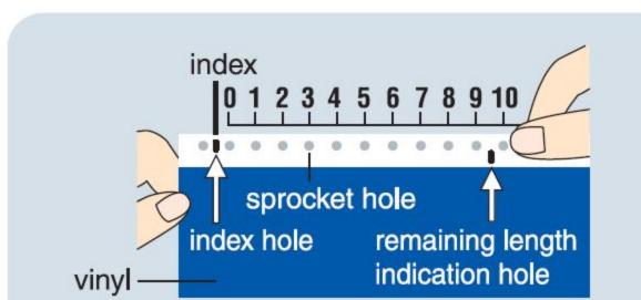
The approximate remaining vinyl length can be checked visually by fitting it to the printed gauge of the box of the vinyl.
